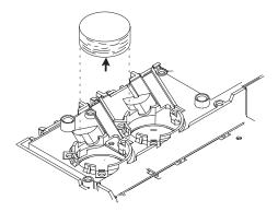
4. Carefully remove the scribed circle of insulation from the oven top to create an opening into the oven, if necessary.
