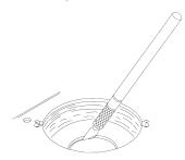
**Method 2:** Pierce the insulation with a screwdriver. Rotate the screwdriver around the circumference of the scribed circle to remove excess insulation.
