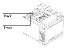
2. Remove the round metal cutout in the front or back inlet position, if necessary. Insert a flat-blade screwdriver into the slot in the cutout and move the screwdriver back and forth until the cutout breaks free from the sheet metal on the oven top.
