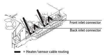
5. Route the stainless steel tubing from the inlet to the flow manifold. Route the tubing along the side of the inlet chassis to the fan bracket. Route tubing from the front inlet outside the bracket and tubing from the back inlet inside the bracket. Route the tubing behind the fan to the flow manifold.
